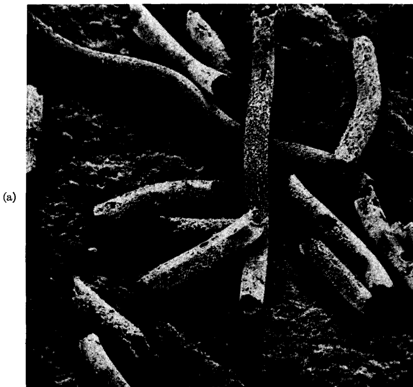
FIG. 1. Scanning electron micrographs of rhodium oxide sheaths separated from the wire core: (a) sheaths magnified 100×; (b) fragment of single sheath, magnified 1000×; (c) fragment of the sheath wall, magnified 10,000×.
